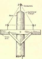
Fig. 104.—Symmetrical arrangement of conductors, three-phase circuit.
